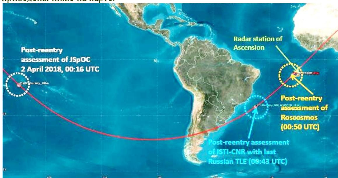
Post-re-entry assessments of Roscosmos and ISTI/CNR, at 10 km of altitude, based on the last Russian TLE, compared with that of JSpOC, based on the last US TLE
